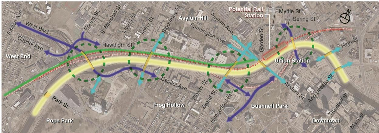
In this alternative, originally proposed in *The HUB Study*, the railroad would be relocated to the north of the highway to allow I-84 to be lowered to, or below, ground level between Park and Trumbull Streets. Local roads crossing the interstate would all be bridges over the highway.
